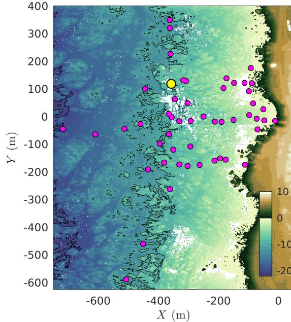
109 FIG. 1. Bathymetry ( $z$  in mean sea-level) as a function of local cross-shore ( $X$ ) and alongshore ( $Y$ ) coordinates.
