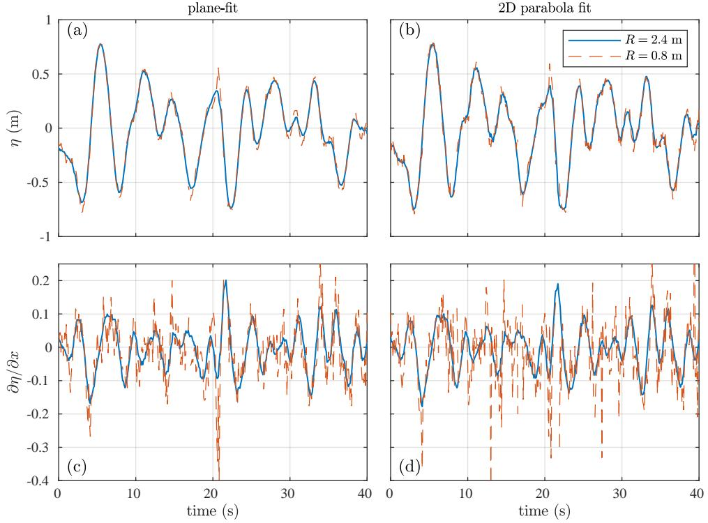
267 FIG. 4. Timeseries of (top, a-b)  $\eta$  and (bottom, c-d)  $\partial\eta/\partial x$  for  $R = 2.4$  m (blue) and  $R = 0.8$  m (orange-dashed)
