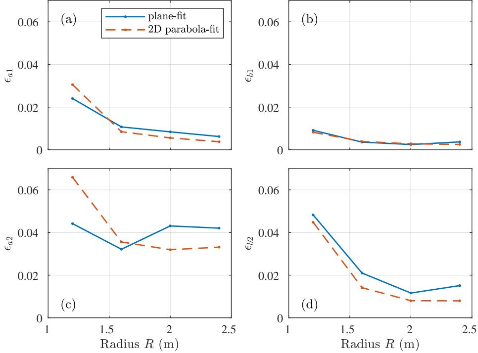
383 FIG. 9. Directional Fourier coefficient errors versus radius  $R$  for (a)  $\epsilon_{a1}$ , (b)  $\epsilon_{b1}$ , (c)  $\epsilon_{a2}$ , and (d)  $\epsilon_{b2}$  based on
