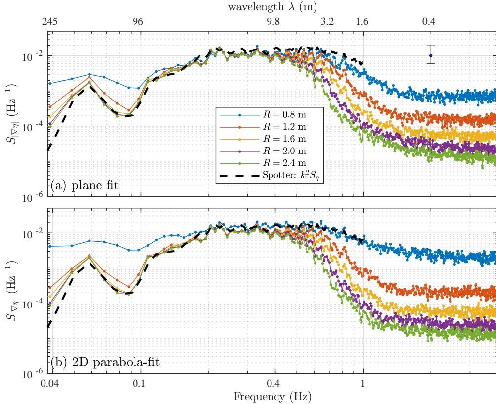
313 FIG. 7. Sea-surface elevation slope spectra  $S_{|\nabla\eta|}$  (6) versus frequency for the (a) plane-fits and (b) 2D parabola-
