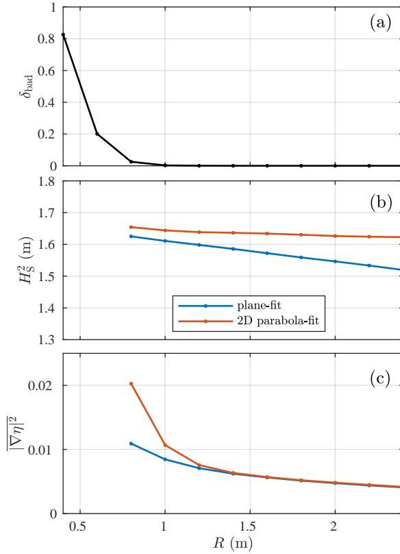
285 FIG. 5. (a) Fraction of time with bad data  $\delta_{\text{bad}}$  (b) squared significant wave height  $H_s^2$  (4), and (c) mean square
