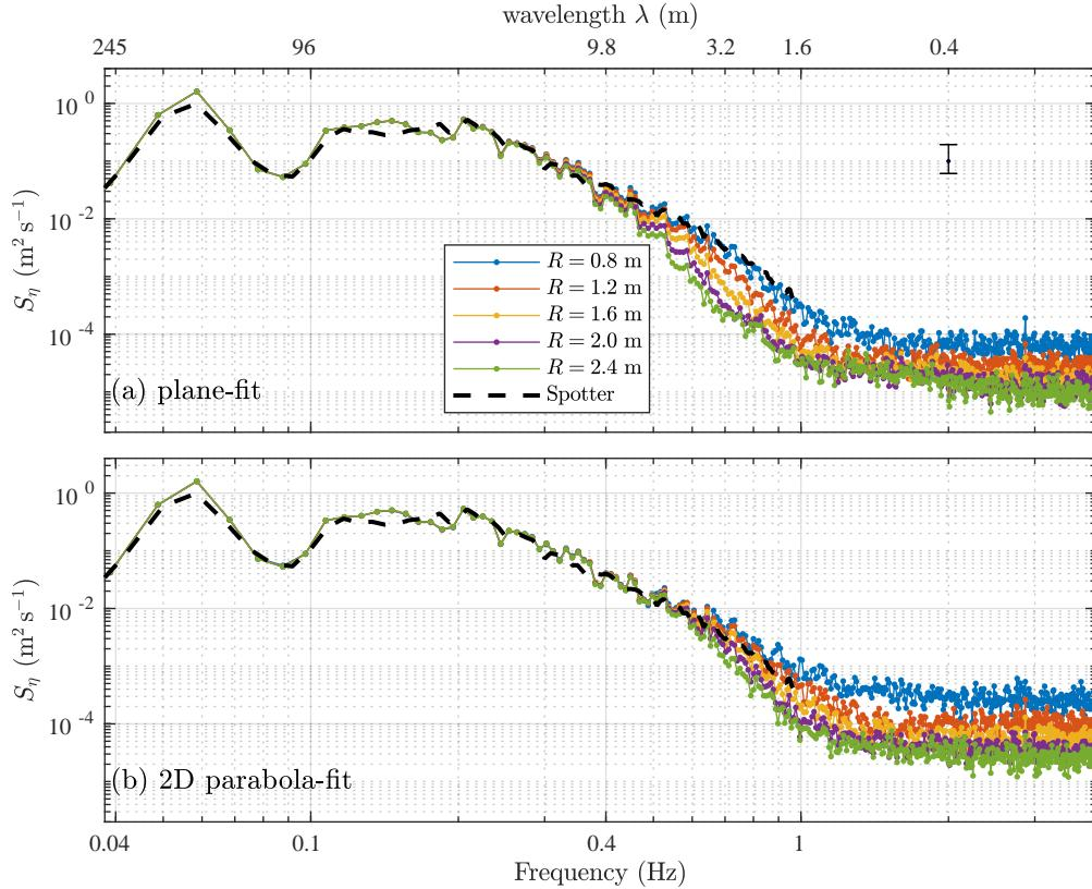
307 FIG. 6. Sea-surface elevation spectra  $S_\eta(f)$  versus frequency for the (a) plane-fit and (b) 2D parabola-fit
