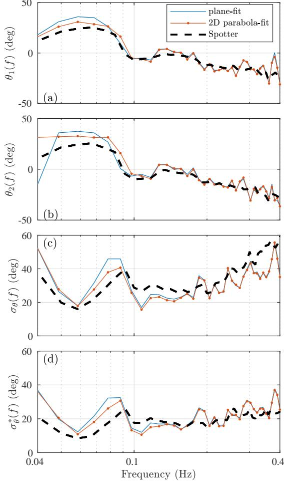
404 FIG. 10. Mean directions (a)  $\theta_1$  (A7) and (b)  $\theta_2$  (A8), and directional spreads (c)  $\sigma_\theta(f)$  (A9), and (d)  $\sigma_\theta^*(f)$
