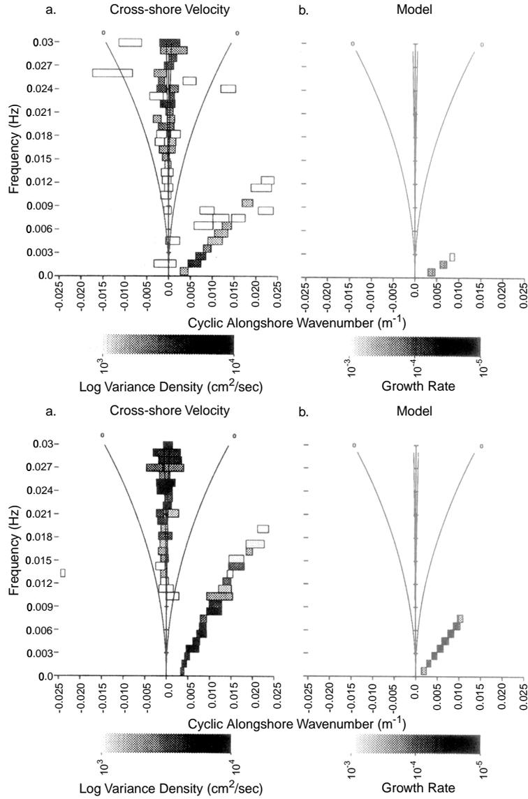
Figure 9: Frequency - Wavenumber spectra of cross-shore velocity in the surfzone at Duck (left) and frequency & wavenumber of the fastest growing disturbance (right) along with the mode zero edge wave dispersion curve. (from *Dodd et al.* [1992]). The top panel corresponds to a period of weak longshore current and current shear relative to the lower panel. (from *Dodd et al.*, [1992]).
