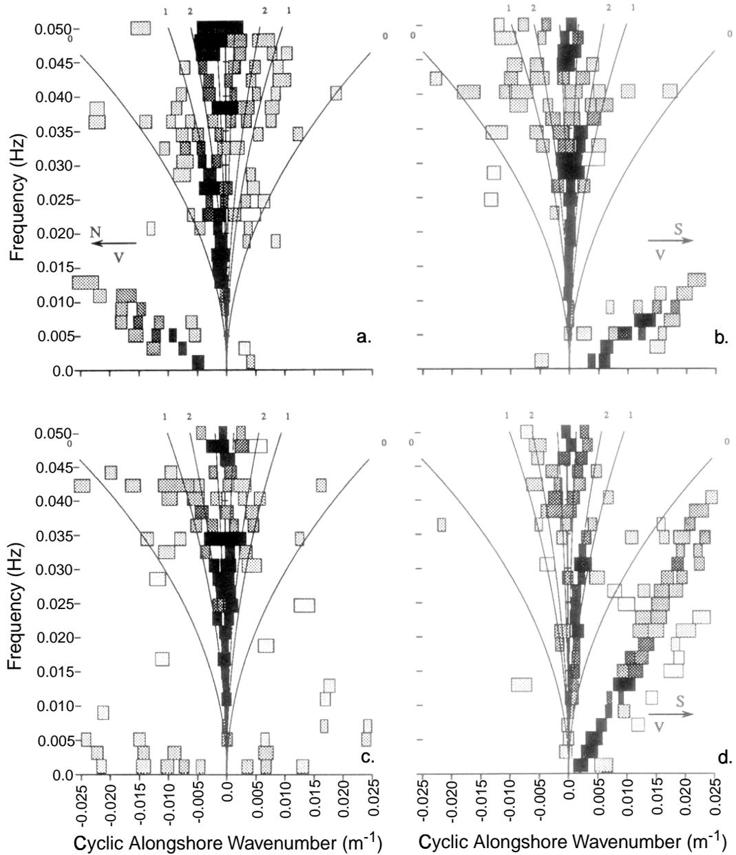
Figure 8: Frequency-wavenumber spectra of cross-shore velocity in the surfzone on four different days. The mode 0,1, & 2 edge wave dispersion curves are superimposed. The direction of the longshore current is also shown. In (c), the longshore current is approximately zero. (from *Oltman-Shay et al.*, [1989])
