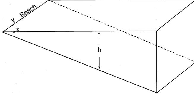
Figure 1: The coordinate system used. Planar beach bathymetry ( $h = \beta x$ ) is shown.
