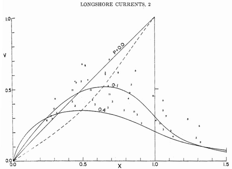
Figure 3: Comparison of  $\bar{v}$  measured by *Galvin & Eagleson* (1965) with the theoretical profiles of *Longuet-Higgins*. The plotted numbers represent  $\bar{v}$  data points. (from *Longuet-Higgins*, [1970])
