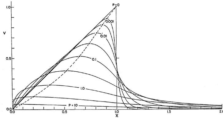
Figure 2: Nondimensional  $\bar{v}$  solutions for a sequence of values of the mixing parameter  $P$ . The breakpoint is at  $x = 1$ . (from *Longuett-Higgins*, [1970])
