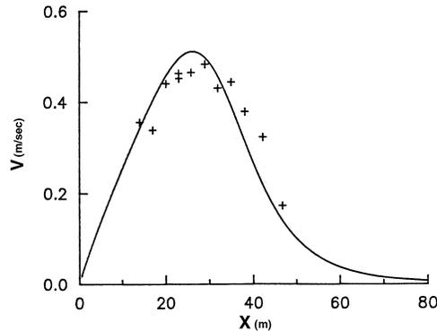
Figure 4: Analytic solution for planar beach with no mixing (solid line) and measurements (+) of  $\bar{v}$  ( 4 Feb 1980, from *Thornton & Guza* (1986)).
