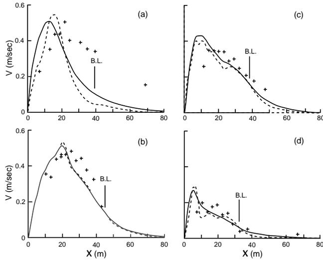
Figure 5: Comparison of modeled and observed  $\bar{v}$  for other days in February. No mixing (solid) & with mixing (dashed). The location of the breaker line is denoted as B.L.
