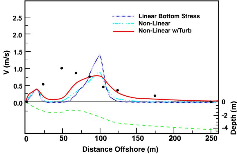
Figure 6: Observations of  $\bar{v}$  (black circles) and model  $\bar{v}$  (three lines) with different parameterizations of the bottom stress. The barred beach bathymetry is shown below. (from Church & Thornton, [1993])
